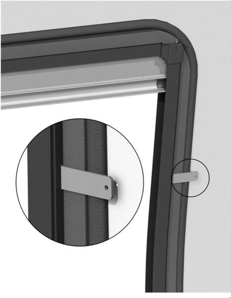
Secure the Rear Screen to the van using 6 type 1 screws and spacer rings.
