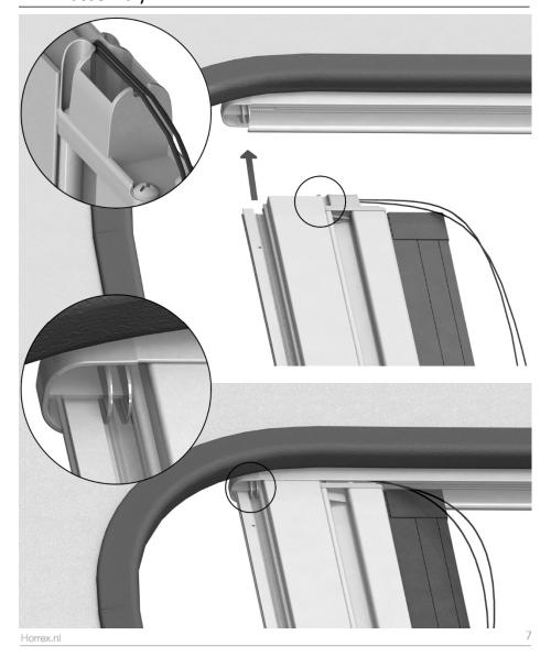
6 Slide the bottom of the cassette and pullbar assembly into the bottom profile.
