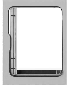
When the cassette and pullbar are vertical fasten the cassette to the bottom profile using 2 type 1 screws.
