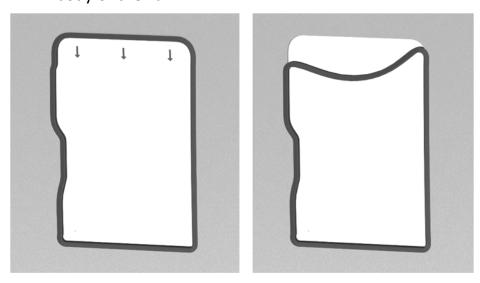
Put the metal clips on the metal edge of the body of the van. Leave an 8mm gap between the topguider and the plastic panel in front.
